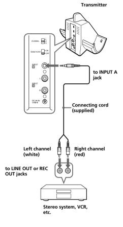
© To connect to TV, etc. If noise occurs when the transmitter is connected to your TV or VCR, set the NOISE FILTER switch to ON.
