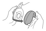
2 Place the new ear pad on the driver unit and insert the edge of the pad into the groove as illustrated.
