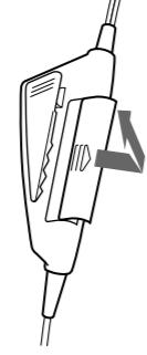
2 Insert one R03 (size AAA) battery by matching the + and - on the battery to the + and - in the battery box.
