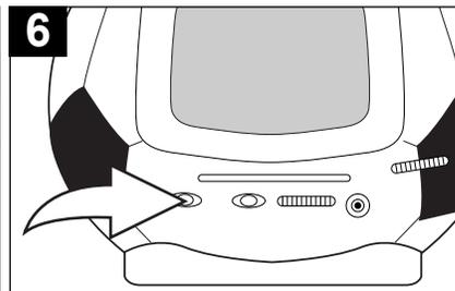
**6** Slide the TV/OFF/RADIO switch to the OFF position to turn the TV off.
