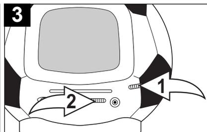
**3** Tune a desired TV station by turning the TUNING control ① and adjust the VOLUME control ② as desired.
