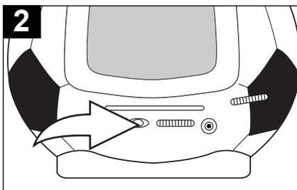
**2** Slide the BAND switch to the desired setting:
