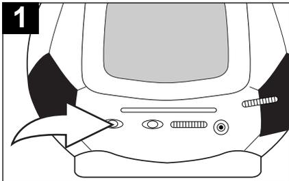
**1** Make sure the EXT/BATT/CHARGE switch is set properly (see page 5). Slide the TV/OFF/RADIO switch to the RADIO position to turn the radio on.
