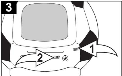
**3** Tune a desired AM or FM station by turning the TUNING control ❶ and adjust the VOLUME control ❷ as desired.
