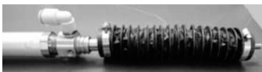
Removal of bellows
