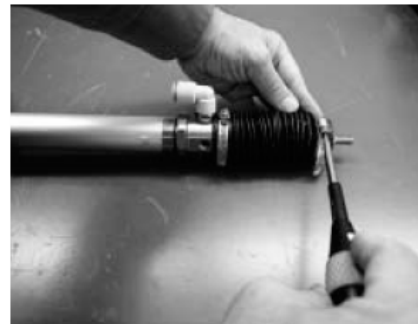
Tightening of front metal fitting
