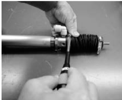
Tightening of rear metal fitting
