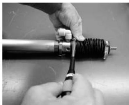
Loosening of rear metal fitting
