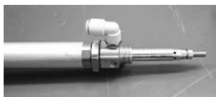
Bellows has been removed
