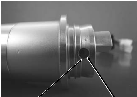
Coupling setscrew hole
