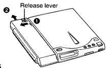
After removing the battery case, remove the batteries from the battery case, then install the new batteries (P. 25).
