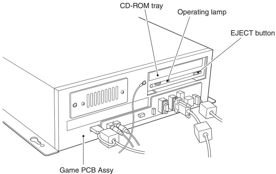
3. Mount the CD-ROM on the tray with the label (print) surface upwards.
