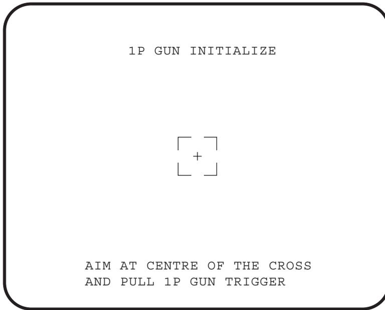
Aim the 1P gun at the cross in the centre of the screen and pull the trigger. The following screen will be displayed.
