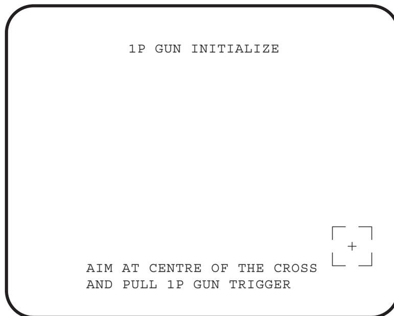
Aim the 1P gun at the cross in the bottom right of the screen and pull the trigger. The following screen will be displayed.
