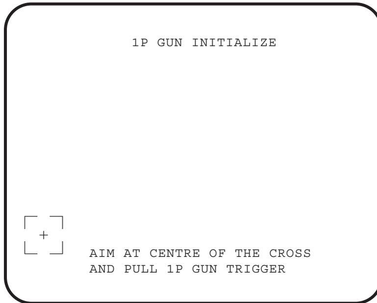
Aim the 1P gun at the cross in the bottom left of the screen and pull the trigger. The screen will revert to showing a cross in the centre of screen. Repeat the above procedures with the 2P gun.
