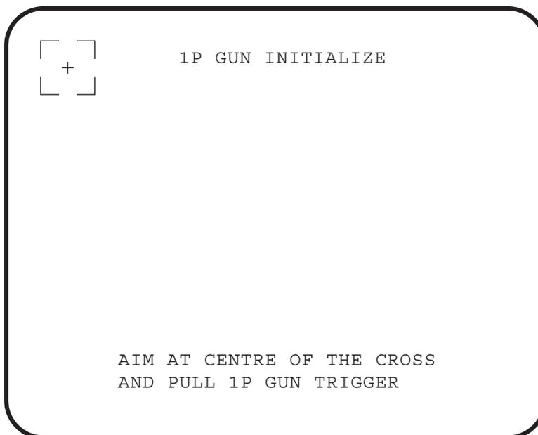
Aim the 1P gun at the cross in the top left of the screen and pull the trigger. The following screen will be displayed.
