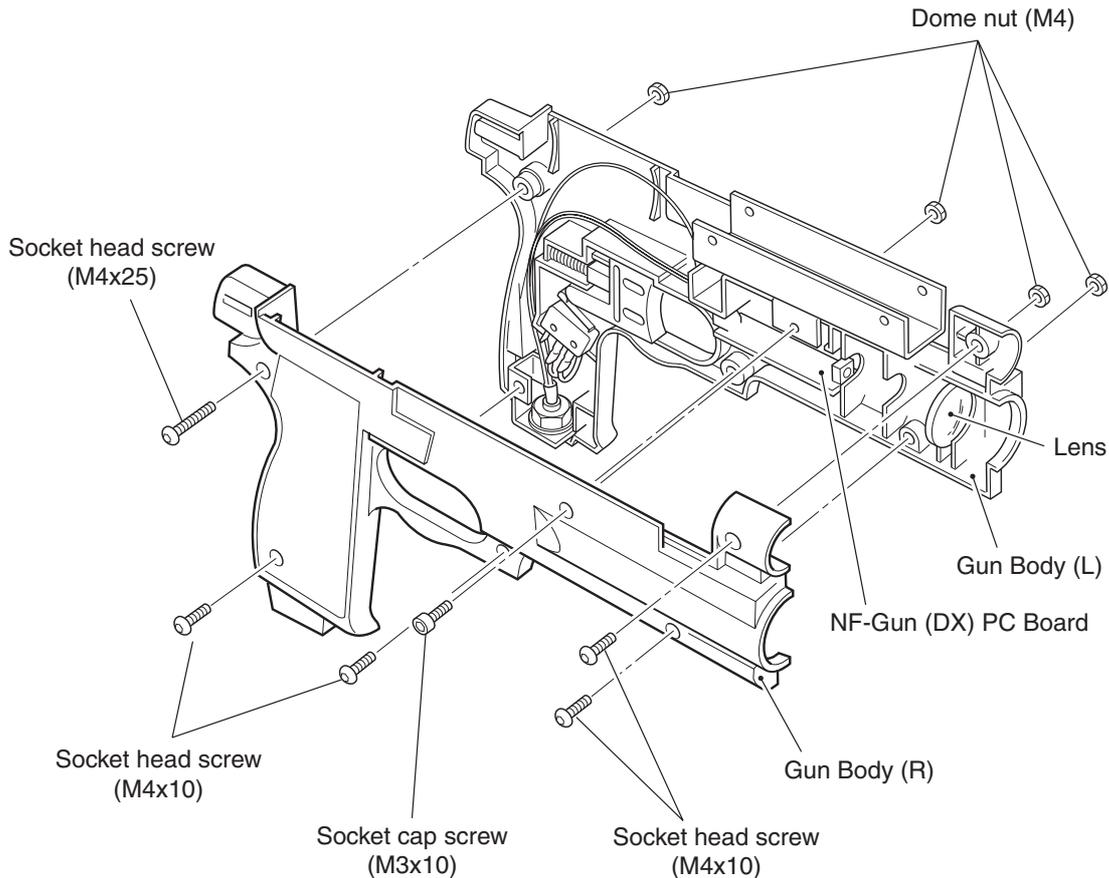
**Note:** When reassembling the Gun Body ensure that the Lens is fitted correctly, (Curved face of lens faces forward.). Failure to fit the lens correctly will prevent the gun from working properly.
