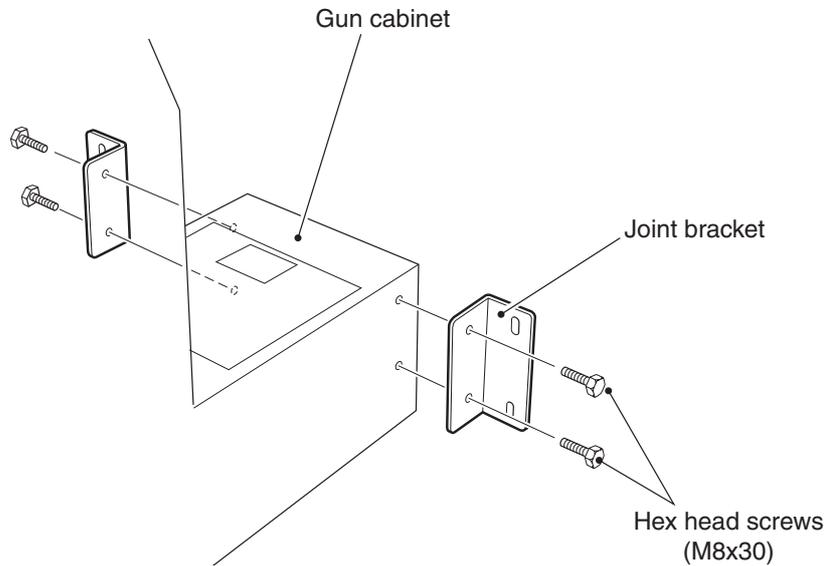
2. Place the Gun Cabinet close to the Monitor Cabinet and connect the connectors.
