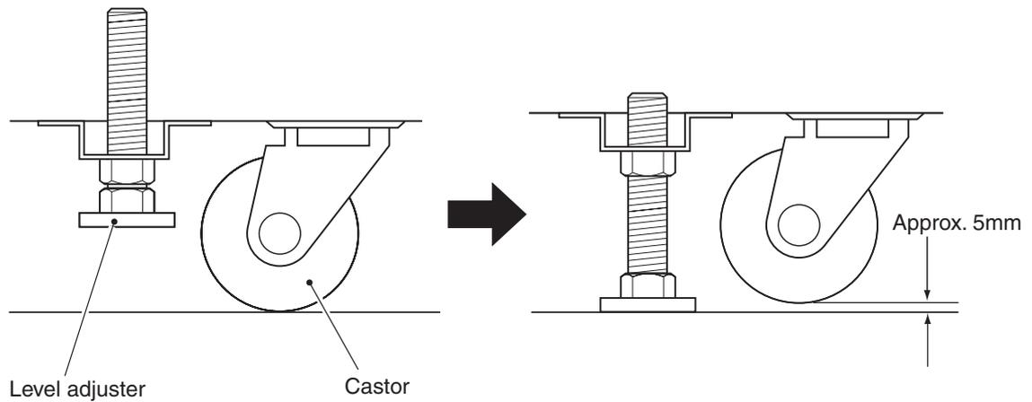
*Note: If the site of this game has a smooth or polished floor, it is recommended that rubber pads are fitted under the Level Adjusters to prevent the game sliding on the floor when in use.*
