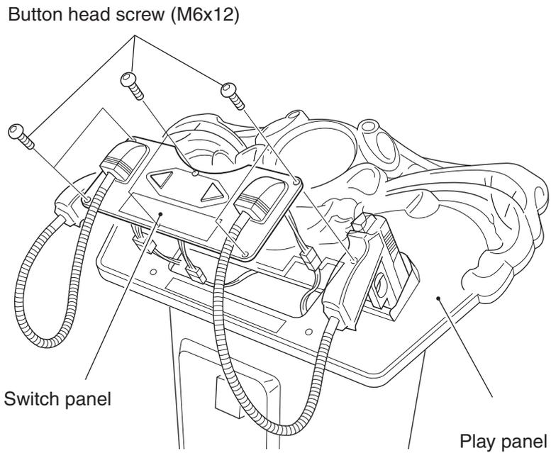
2. Disconnect the connectors and remove the Switch Panel Assy.
