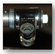
3. Starting with the bottom clevises, place a 5/8 bolt through each clevis (Scotts imprint facing up) using 1 washer under the bolt. With the bolt through the clevis, place 3 washers on the bolt. When you are done you should have each clevis sandwiched between 4 washers with 3 on the inside and 1 on the outside. Thread the bolt in to the Crossmember and torque to spec.
