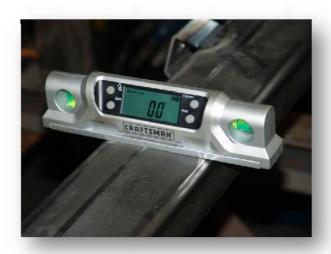
7. Tack the cross-member in place and double check your level. When you are satisfied with the fit and level, weld the cross-member into place.
