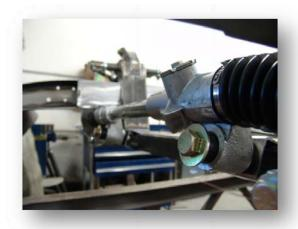
4. To bolt the rack to the spindles at this point, you only need to be "close". This will be adjusted during the alignment process. Start by holding the spindles as close to straight as possible. Thread in, or thread out the outer tie rod on until it lines up with the steering arm. Place the tie rod into the steering arm and secure with the castle nut. Do not tighten yet as this will need to come back off for alignment.
