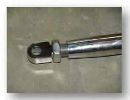
2. Step two is to assemble all 8 Stainless clevises and bolt them to the Crossmember. You will need (8) clevises with "Scotts" imprint, (8) bushing and sleeve packs, (32) 5/8" SAE washers, and (8) 5/8"-18x3-1/2" grade 8 yellow bolts. Insert (1) sleeve and (2) bushing halves into each clevis. Each clevis will also use 4 washers and 1 bolt.
