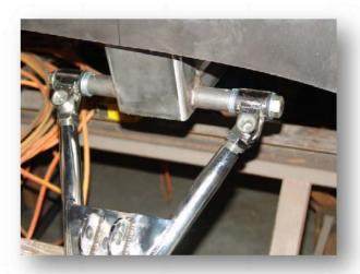
5. Next you will need (2) coilover shocks, (4) 5/8-18x3" grade 8 yellow bolts, (8) 5/8 grade 8 yellow washers, and (4) 5/8-18 nyloc nuts. Install the coilover shock into the upper shock mount using (1) 5/8 bolt, (2) 5/8 washers, and (1) 5/8 nyloc nut. After the upper mount is tightened, attach the shock to the lower a-arm using the same hardware as the upper mount.
