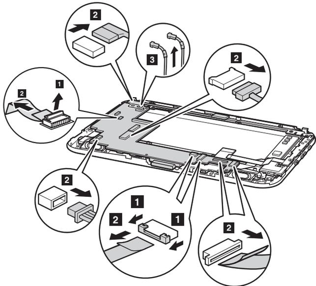
Figure 5. Removal steps of system board (continued)
