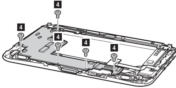
**When installing:** Make sure that all the connectors are attached firmly.
