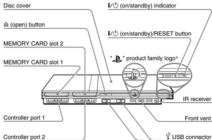
\* The "PS" product family logo can be rotated to match the horizontal or vertical positioning of the console.
