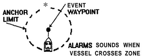
The first task, when entering an anchor watch alarm, is to press the **EVENT/6** key as you drop anchor to store your present position as a waypoint. Make a mental note of the **EVENT** memory # (number). The number appears for approximately 3 seconds on the **display** and certainly is the last used waypoint. If you miss seeing the number, just check the **waypoint** list. The stored Event will be the highlighted **waypoint** on the list.
