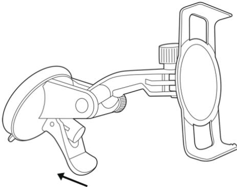
1. Clean that part of the windscreen to which you want to secure the cradle. The windscreen must be dry and free of dirt and grease.
