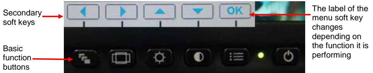
Figure 5 Soft key buttons
