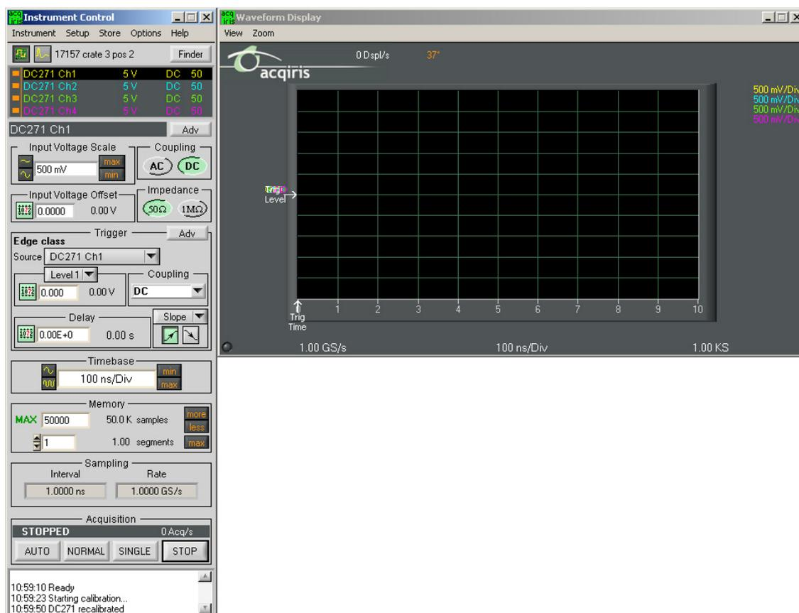
AcqirisLive displays two independent windows, a control window and a display window. The control window contains functions that allow you to manipulate the acquisition parameters of the card. In order to display an acquired waveform, connect a signal to the input, and then select the Auto acquisition mode at the bottom of the control panel. A waveform should appear in the display.
