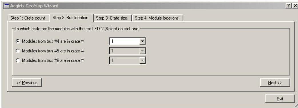
Selecting a row will cause all of the LED's of modules in that Bus to be turned on RED. This should make it easy to identify which crate the modules are in.
