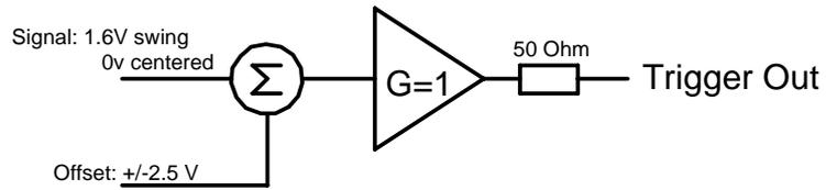
The output swing is 1.6 V ( $\pm$ ) when unloaded and 0.8 V when terminated on 50  $\Omega$ . The rise and fall times are 2.5 ns typical. The offset can be adjusted, by software control in the range  $[-2.3 \text{ V}, +2.3 \text{ V}]$  unloaded, or  $[-1.15 \text{ V}, +1.15 \text{ V}]$  into 50  $\Omega$ . The maximum output current capability is  $\pm 15 \text{ mA}$ . As the output is retro-terminated, it is possible to drive a 50  $\Omega$  line unterminated (HiZ) without loss of performance.
