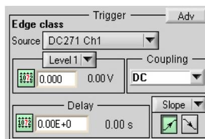
The *Coupling* section also contains a selection for AC or DC coupling. AC coupling on the trigger sets the trigger circuit to an AC Low Frequency Reject mode.
