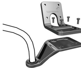
5. Screw the Holder to the Adhesive Mount using four of the small screws included with the mounting kit.
