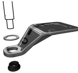
**Note:** The washers help to prevent the mirror mount from moving or from being damaged. Select the diameter of the washers according to the diameter of the bolt hole.
