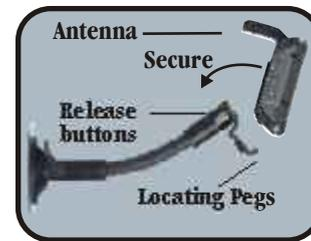
Fig 2: Secure unit to bracket
