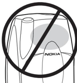
While in a call, hold the phone to your ear, placing your finger tips on the Nokia badge at the mid-center of the back cover (located below the antenna area on the back of your phone).
