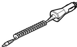
The input voltage range is from 11 V to 32 V DC, negative grounding. Avoid prolonged charging with the Rapid mobile charger (LCH-12) when the car engine is not running; this could cause your car battery to drain. Note also, that in some cars, the cigarette lighter plug is not provided with electricity if the ignition is not switched on.
