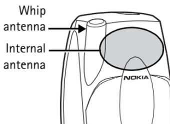
As with any other radio transmitting device, do not touch either of the two antennas unnecessarily when the phone is switched on. Contact with the antenna affects call quality and may cause the phone to operate at a higher power level than otherwise needed. Not touching the antenna area during a phone call optimizes the antenna performance and the talk time of your phone.
