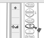
3 Select the fan speed by pressing the FAN button one or more times until the required setting is displayed:
