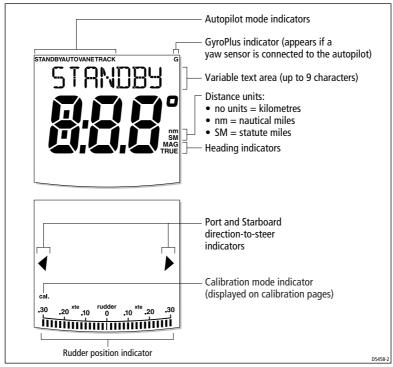
The bar graph at the bottom of the screen indicates the current position of the rudder, as measured by the rudder position sensor.
