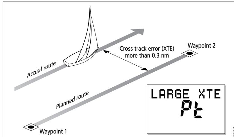
Cross track error (XTE) is the distance between the current position and a planned route. The SmartPilot receives the cross track error information
