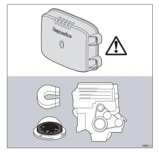
The receiver should be installed a minimum of 3 ft. (1m) away from an engine, compass or any magnetic device.
