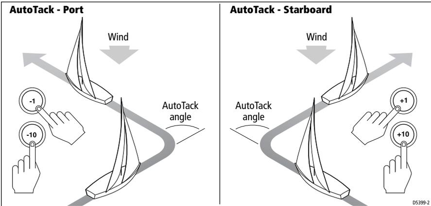
**Note:** *If you have set the vessel type to SAIL BOAT, you can adjust the default AutoTack angle in User Calibration (see page 23).*
