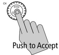
4. When the NAME entry is complete, push in the CH knob to accept it.
