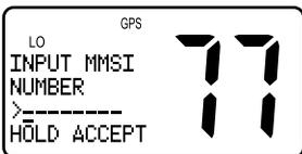
3. To enter the MMSI ID number, rotate the CH knob to select the digits using the same technique described in *Adding an Entry on page 59*.
