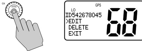
3. Rotate the CH knob until the arrow is pointing to DELETE.
