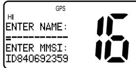
3. Use the CH knob to enter the NAME that you wish to have associated with this MMSI ID number. Rotate the CH knob to select each character and then push in the knob to accept it.
