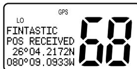
**Note:** Only the last position is saved. The next received position will overwrite the existing position data.
