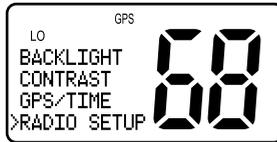
3. Push the CH knob to accept. The Radio Setup screen appears.
