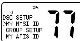
2. Push the CH knob to accept. If an existing MMSI ID is stored, the value appears. If the MMSI ID is blank, dashes appear, indicating that one has yet to be entered.
