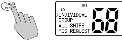
2. Rotate the CH knob until the arrow points to CALL LOG
