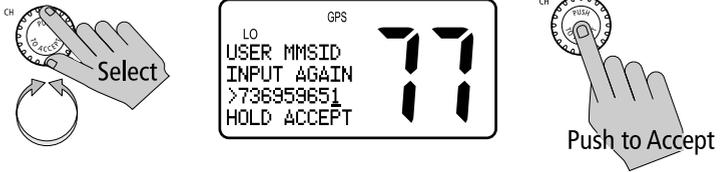
6. When complete, **press and hold** the CH knob to accept.
