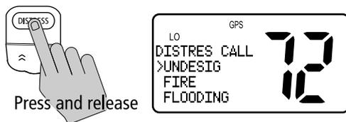
2. Rotate the CH knob until the arrow points to the type of Distress you wish to designate.
