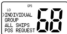
2. Rotate the CH knob until the arrow points to ALL SHIPS.
