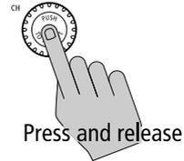
You can also press the microphone UP/ DOWN keys to select each character and then press the microphone HI/LO key to accept.
