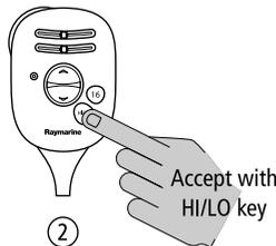
4. When complete, **press and hold** the CH knob to accept.
