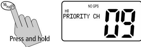
If on primary Priority CH16, **press and hold** the 16/PLUS for greater 3 seconds to switch to the Secondary Priority (PLUS) Channel at HI power. The default is CH 9.
