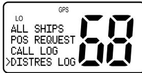
3. Push the CH knob to select the Distress Log. Entry 01 (the most recent call) appears first with call type and position data. The screen then flashes to display the nature of the distress and time of the call.
