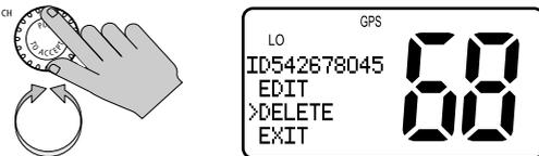
4. **Press and hold** the CH knob. The entry is removed.
