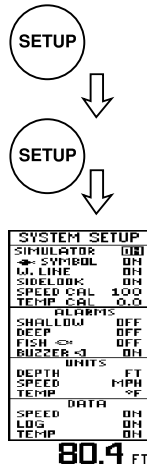
Fig. 4-9 Reaching the System Setup Display
