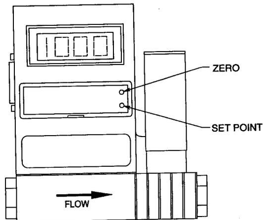
The versatile FMA-1900 product digitally displays the mass flow rate directly in engineering units or percent of full scale.
