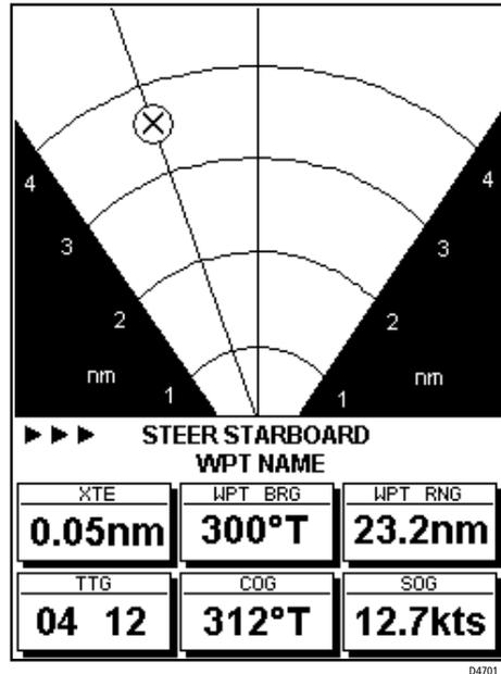
The line to the waypoint symbol is shown at an angle equal to the difference between the COG and the Bearing to Waypoint. The waypoint symbol is the symbol of the target waypoint as seen on the chart.
