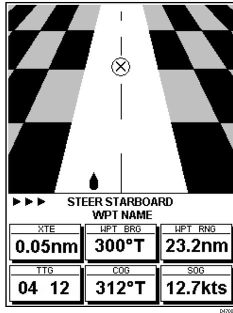
The 'runway' represents a 0.3nm width with the vessel symbol shown at the bottom. Bearing to Waypoint, Distance to Waypoint, Time to Go (TTG), Course Over Ground (COG) and Speed Over Ground (SOG) are also shown. Time to Go is calculated on the basis of distance to destination and Speed Over Ground (SOG) towards the destination.
