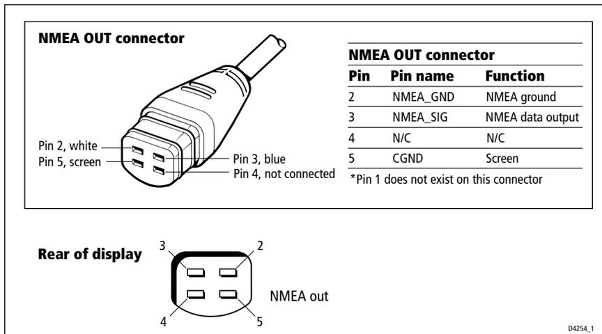
Figure 6-13: NMEA Output Connector
