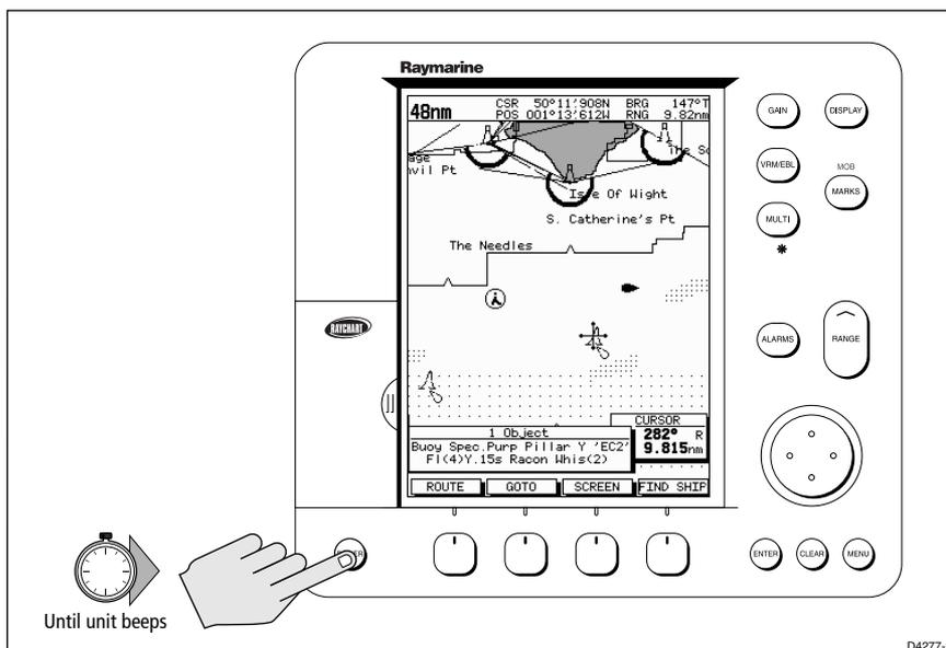
Figure 2-1: Switch On - Chart Mode
