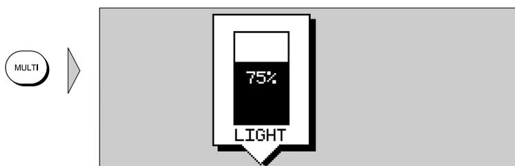
2. The **LIGHT** soft key indicates the brightness level, use the trackpad (up or down) to increase or decrease the setting. You can press and hold the trackpad to change the setting more rapidly. The brightness level is adjusted as you change the setting.
