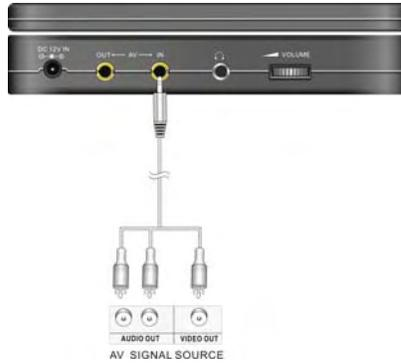
1. Connect the audio/video cable to the GPS AV In jack and to the external AV signal source. Make sure that you match the color-coded ports and plugs while connecting audio and video cables.
