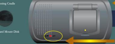
Switch "ON" on the back of the device
