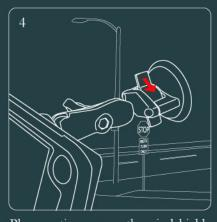
Place suction cup on the windshield and move the clip over to the right to create the suction. It is
