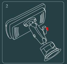
Tighten the clamp by turning the knob The GPS should now be connected
