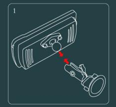
Loosen the knob on the side of the clamp turning it counter clock-wise. Attach it to the GPS
