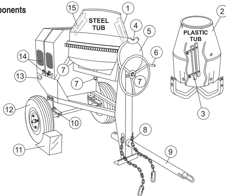
1. **Steel Mixing Drum** — The MQ Whiteman WC-62S uses a 6 cu. ft. **steel** mixing drum. This drum is to be used for mixing of concrete. Always clean the drum after each use. **DO NOT** use this mixing drum for the mixing of volatile liquids.
