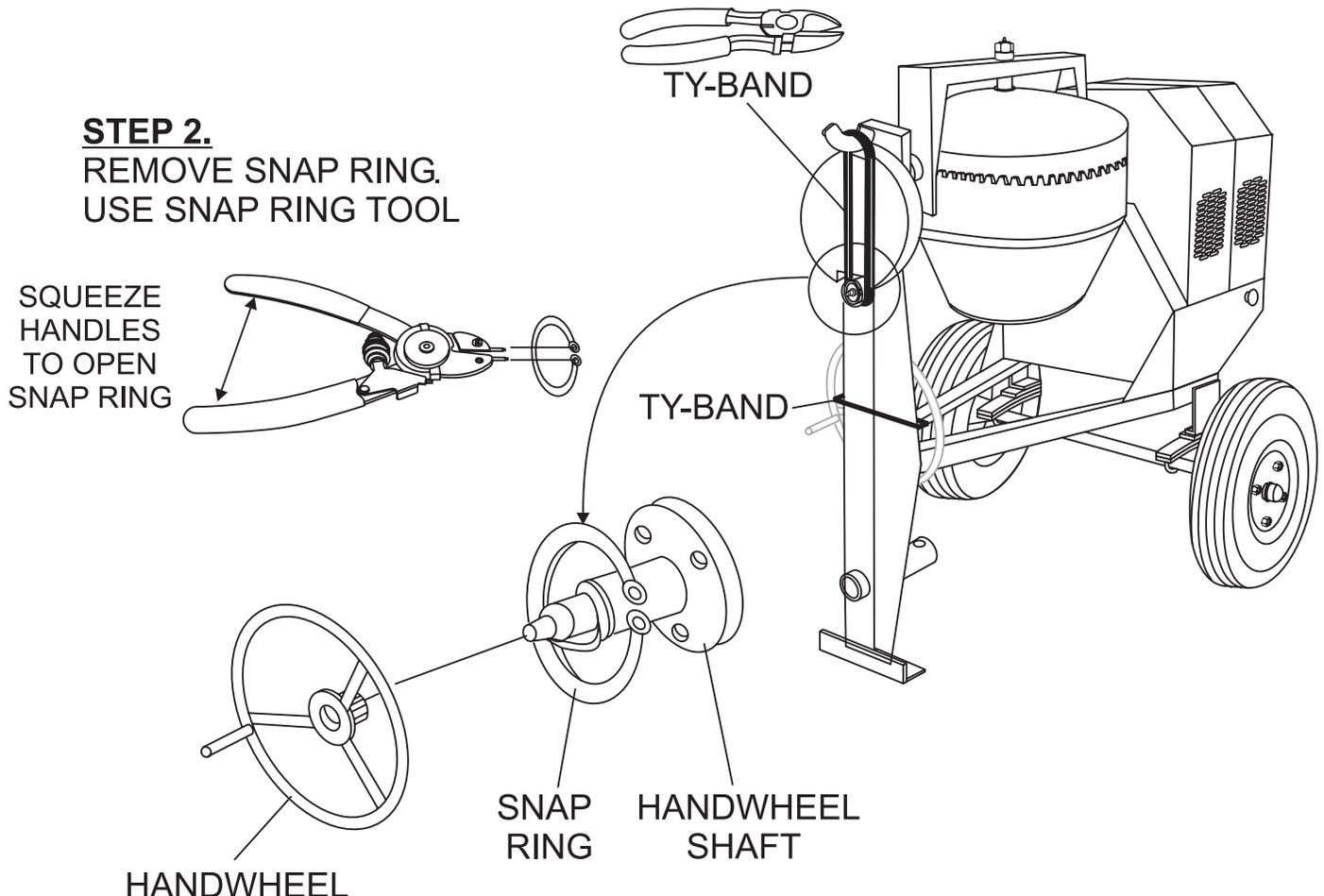
Figure 4. Handwheel Assembly
