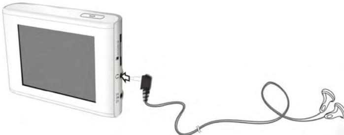
When earphone is connected, the speakers will automatically turn off.
