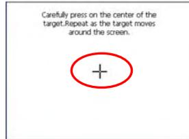
This item is used to calibrate the sensitivity of the touch screen. Tap the center of “+” as it moves around the screen. If you touch the center of “+” every time, it will disappear after having moved through a cycle (center→top left→bottom left→bottom right→top right). Tap the screen to return to the settings menu.
