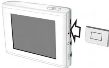
To remove the card, gently press the card in with your fingernail. The card unlocks and protrudes slightly. Then remove the card.
