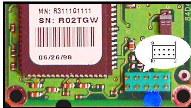
Figure 1 - Oncore™ GPS 10 Pin Connector Pinout
