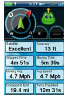
The Dashboard Screen displays a small compass and up to eight customizable data fields. The data fields displayed are customizable (see *Customizing the Data Fields*).
