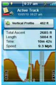
The Altimeter Screen displays detailed elevation information using the GPS signal. The area on the graph can be expanded by selecting the icon in the lower right corner and defining the area to be used. Also a line can be moved along the graph to pinpoint an exact point on the graph and display detailed information on that point.
