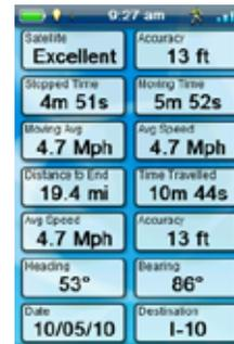
The Data Only Screen displays the most number of data fields available to be viewed at one time in the receiver. Up to 12 customizable data fields can be viewed at one time. The data fields displayed are customizable (see *Customizing the Data Fields*).
