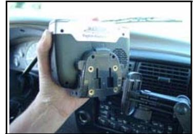
Press the windshield mount to the glass and slide the locking lever toward the glass.
