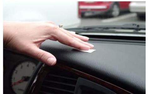
2. Peel the paper cover off of the adhesive backing.
