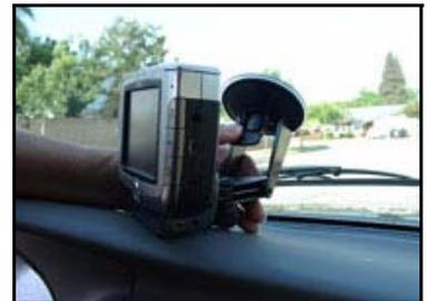
Plug the power cable and FM antenna into the Magellan RoadMate 6000T as shown. Use the suction cups to position the FM antenna along the windshield.
