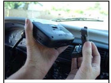
Slide the windshield mount onto the back of the cradle.
