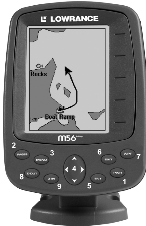
Lowrance M56 Sonar, front view, showing screen and keyboard. (A close-up of the keyboard can be found at the beginning of Sec. 6)
