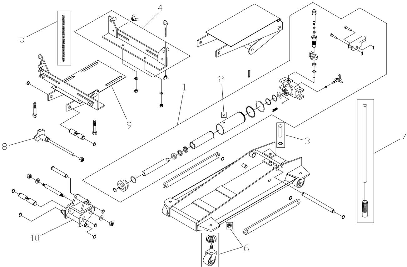
Figure 2 - Replacement Parts for Model 41100
