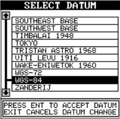
The WGS-84 label is highlighted. To change it, simply press the up or down arrow keys until the desired datum is highlighted, then press the ENT key. This selects the datum and erases the datum menu. The GlobalMap 12 is now using the datum you selected.
