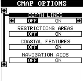
These menu items let you turn the depth lines, restriction areas, coastal features, and marine navigation aids off or on. Highlight the desired feature, then press the right or left arrow key to change them. Press the EXIT key when you're finished.
