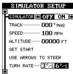
To change either the track or speed, highlight the one you want to change, then press the right arrow key. Use the up and down arrow keys to change each number, then use the left and right arrow keys to select the other numbers that you wish to change. On the example at right, the speed is changed from 100 m.p.h. to 30 m.p.h.. When the numbers are correct, press the EXIT key.
