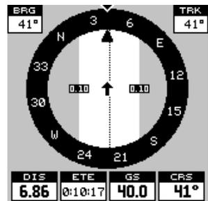
The numbers on either side of the center arrow show the cross track error range. In other words, (using the screen at right as an example) if the arrow crosses the dark band on either side, you are .10 miles to the left or right of the desired course.
