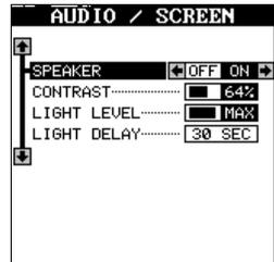
The backlights brightness is also adjustable. To do this, highlight the "Light Delay" label. Now press the left or right arrow key until you have the lights at the desired level. Press the EXIT key when you're finished. The default light level is maximum.
