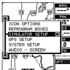
If you simply press the right arrow key, turning the simulator on, the GlobalMap 12 will start from your present position and follow a track of 0° at 100 miles per hour.
