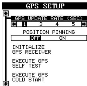
This is the GPS initialization screen. The position, altitude, time, and date the GPS receiver is currently using to find the satellites is shown at the bottom of this screen. Changing these values to your local position and time will speed the position lock.
