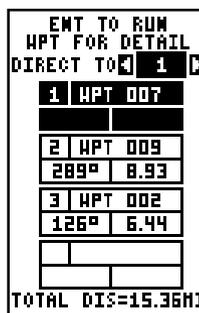
The "Start RTE Auto" label is highlighted. This starts the navigation along the leg of the route that is closest to your present position. On the screen shown at right, waypoint number 7 is the closest to the present position. If you want to start the route with a different waypoint press the right arrow key until the desired waypoint number appears.
