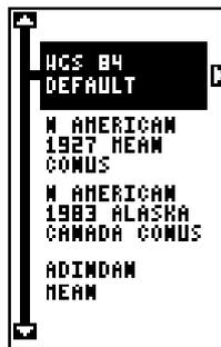
The WGS-84 label is highlighted. To change it, simply press the up or down arrow keys to highlight the desired datum, then press the ENT key. This selects the datum and erases the select datum menu. To erase the menu without changing the datum, simply press the EXIT key.
