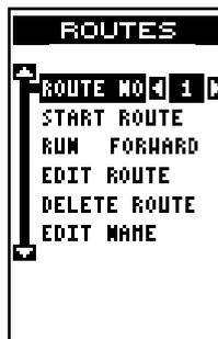
To follow a route, first select the route number that you wish to follow by highlighting the "Route No" label, and pressing the left or right arrow keys until the desired route number appears. In this example we're using route number one. Now highlight the "START ROUTE" label and press the right arrow key. The screen shown at right appears.
