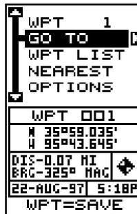
Highlight the "WPT" label at the top of the screen. Press the right or left arrow keys until the desired waypoint number appears that you wish to save your present (or cursor) location under. When it does, highlight the "Options" label and press the right arrow key. The screen shown at right appears.
