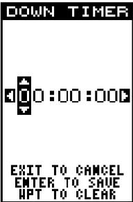
(Note: When the countdown timer reaches zero, it begins counting *up* until you press the EXIT key. This tells you how long it's been since the alarm sounded.)
