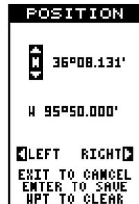
sition and change it using the up and down arrow keys. When you're ready to save this position and return to the waypoint screen, press the ENT key. Press the EXIT key to erase the menus and return to the navigation, plotter, or windows screen. Note: You can also use this method to change the position of an existing waypoint.
