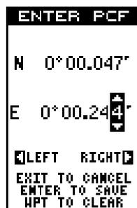
After you've entered the latitude/longitude correction, press the ENT key to accept it. The GlobalNav 212 erases the PCF entry screen and returns to the navigation or mapping screens with the correction factor applied.
