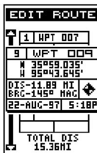
This screen shows the waypoint's name, number, creation time and date, icon, position, distance, and bearing from your present position. When you're finished viewing this information, press the EXIT key to erase it.
