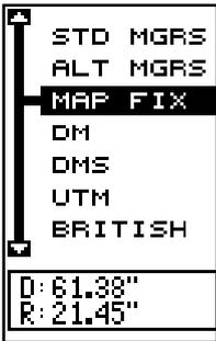
Finally, press the EXIT key to erase this menu. Now highlight the Position Format label and press the right arrow key. Select Map Fix from the list and press the EXIT key. All position information now shows as a distance from the reference point you entered and saved as a waypoint earlier.
