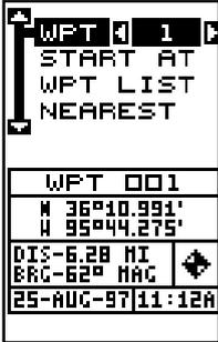
You can select any waypoint as the simulator’s starting point. Select the starting point by pressing the right arrow key on the “WPT#” label until the desired starting waypoint number appears. Now highlight the “Start At” label and press the right arrow key. The GlobalNav 212 returns to the Simulator Setup menu using the waypoint you specified as the starting waypoint.
