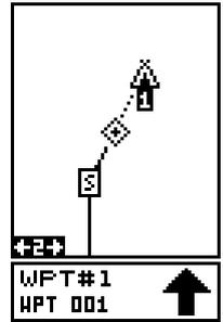
The Z-IN and Z-OUT keys zoom-in and out all plotters to enlarge or reduce their coverage area. The available ranges are: 0.1, 0.15, 0.2, 0.3, 0.4, 0.6, 0.8, 1, 1.5, 2, 3, 4, 5, 6, 8, 10, 15, 20, 30, 40, 60, 80, 100, 150, 200, 300, 400, 600, 800, 1000, 1500, and 2000 miles. Pressing both the Z-IN and Z-OUT centers the cursor's position on the plotter screen.
