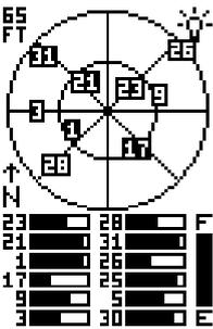
The GPS receiver is tracking satellites that are surrounded by a black box. If the satellite number is not surrounded by a box, then the receiver hasn't locked onto that satellite and it isn't being used to solve the position.
