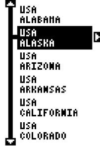
Using the quick initialization method loads a position that's close to yours into the GPS receiver. It should now have position, time, and date, thereby giving it the data it needs to determine which satellites are in view. Once the satellites are known, the receiver searches for only those satellites, making a lock much faster than an auto search method.
