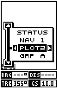
Press the right arrow key while the above menu is showing to switch between different versions of each mode. When the desired screen appears, press the EXIT key to erase the menu.
