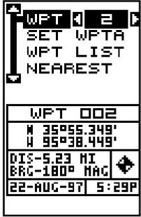
This screen is virtually identical to the waypoint screen. Select a waypoint using the waypoint number, from the waypoint list, or the nearest waypoint list. After selecting the waypoint, highlight the “SET WPT A” label and press the right arrow key. The unit returns to the distance between waypoints screen.
