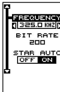
These menus select the beacon receiver's frequency and bit rate (in bits per second). To change one of these settings, simply highlight the menu item you wish to change, then press the right or left arrow key until the desired number appears. Press the EXIT key when you're finished.
