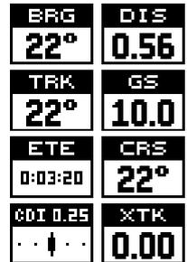
This screen is composed of eight digital boxes. Track (TRK) and ground speed (GS) are all that show if you're not navigating to a waypoint. If you are navigating to a waypoint, then bearing (BRG), distance to waypoint (DIS), estimated time en route (ETE), course (CRS), cross track error (XTK), and the CDI also operate. See below for more information on the CDI.
