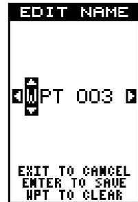
Press the up or down arrow keys to select the first letter in the name. Press the right arrow key to highlight the next position in the name. Repeat this sequence until you've entered all of the letters in the waypoint name. Press the ENT key to accept this name, the WPT key to erase all characters in the name, or the EXIT key to leave this screen without saving any changes.
