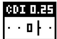
in the center. If you drift off course to the left, the line moves to the *right*. This signifies that you need to steer to the right to get back on course. This is called “chasing the needle”. If you steer towards the line (needle), you’ll always be heading in the correct direction to get back on course.
