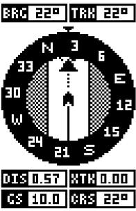
Lines on either side of the present position show the current cross track error range. Cross track error is the
