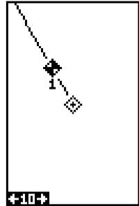
Every time you save a waypoint, the date and time are logged along with the position data. Its icon is also placed on the plotter as shown at right. In this case, waypoint number one was assigned when the position was saved.
