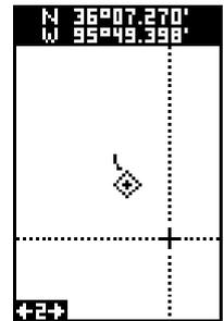
To turn the cursor on, simply press the arrow key in the direction you want the cursor to move. This lets you view areas on the plotter that are away from your present position. The cursor's latitude and longitude show at the top of plot-1's screen. The zoom-in and zoom-out keys work from the cursor's position when it's active - not the present position. You can zoom in on any detail, anywhere. The cursor can also place icons and waypoints.
