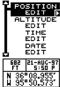
To change a number in the position, highlight it using the right arrow key, then use the up or down arrow key to change its value. The left arrow key acts as a backspace. When the position is correct, press the ENT key.
