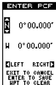
To change the PCF offset, first press the MENU key, then highlight the "GPS Setup" label and press the right arrow key. Now highlight the "Set PCF Offset" label. Finally, press the right arrow key again. A screen similar to the one above right appears.
