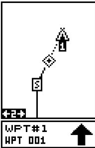
Plot-3 (see at the top of the next page) is similar to plot-2. The major difference is the steering arrow and waypoint information at the bottom of the screen. When you navigate to a waypoint, the waypoint's name and number show at the bottom of this screen. The steering arrow always points in the direction to the waypoint.
