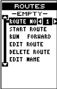
At the bottom of this menu is the “Edit Name” label. If you wish to name the route, highlight that label, then press the right arrow key. Use the arrow keys to name the route, (you can use up to eight characters in the name) then press the ENT key when you’re finished.
