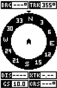
When navigating to a waypoint, Nav screen number one looks like the one at right. Bearing to the destination waypoint is in the box in the upper left corner. Bearing is also shown by the large arrow pointing up towards the compass, above the present position arrow. Distance from the present position to the waypoint (DIS) shows beneath the compass on the lower left side of the screen.
