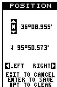
Press the EXIT key to erase the full initialization menu. The unit will use the data you entered to find the satellites that are currently in view. The receiver should lock onto them and show a position within a few minutes.
