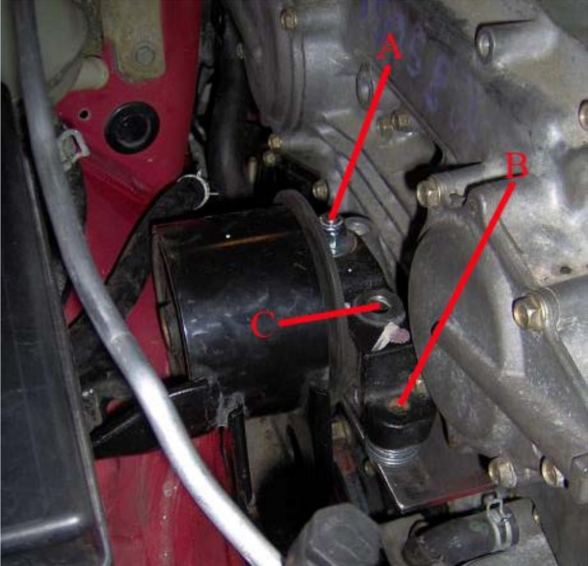
**A & B- Add/Remove shims from between the QR engine mount and the adaptor plate, as needed to get your engine as level as possible. Remember, start with 2-3. That should get you very close. You may also have to use a few washers on the underside of the stud on the hole marked "B", as the stud is a decent length. There should be plenty of washers to accommodate you.**
