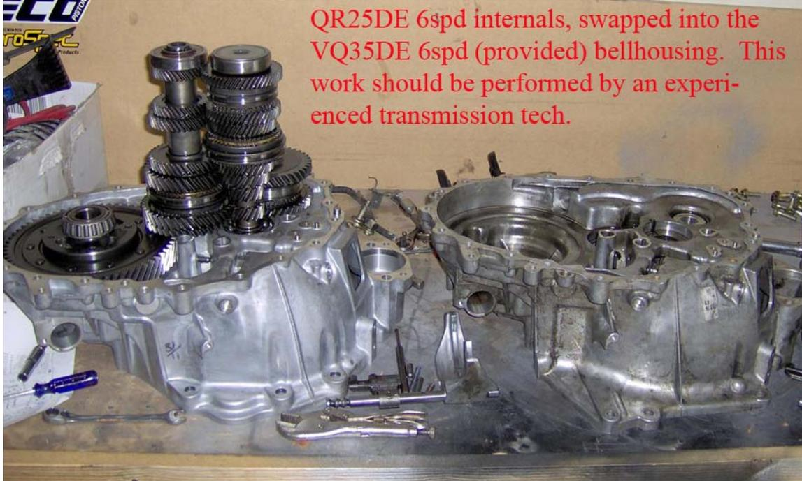
The VQ bell-housing is shown on the left side, with the QR internals already installed. The old QR bell-housing is shown on the right. It is important to check clearances and re-shim the main/input shaft and gear stacks if necessary. As stated, please use the Factory Service Manual, if you are have the knowledge/tools to perform this part of the swap. If you do not, then please consult a local transmission specialist to take care of this part of your swap.
