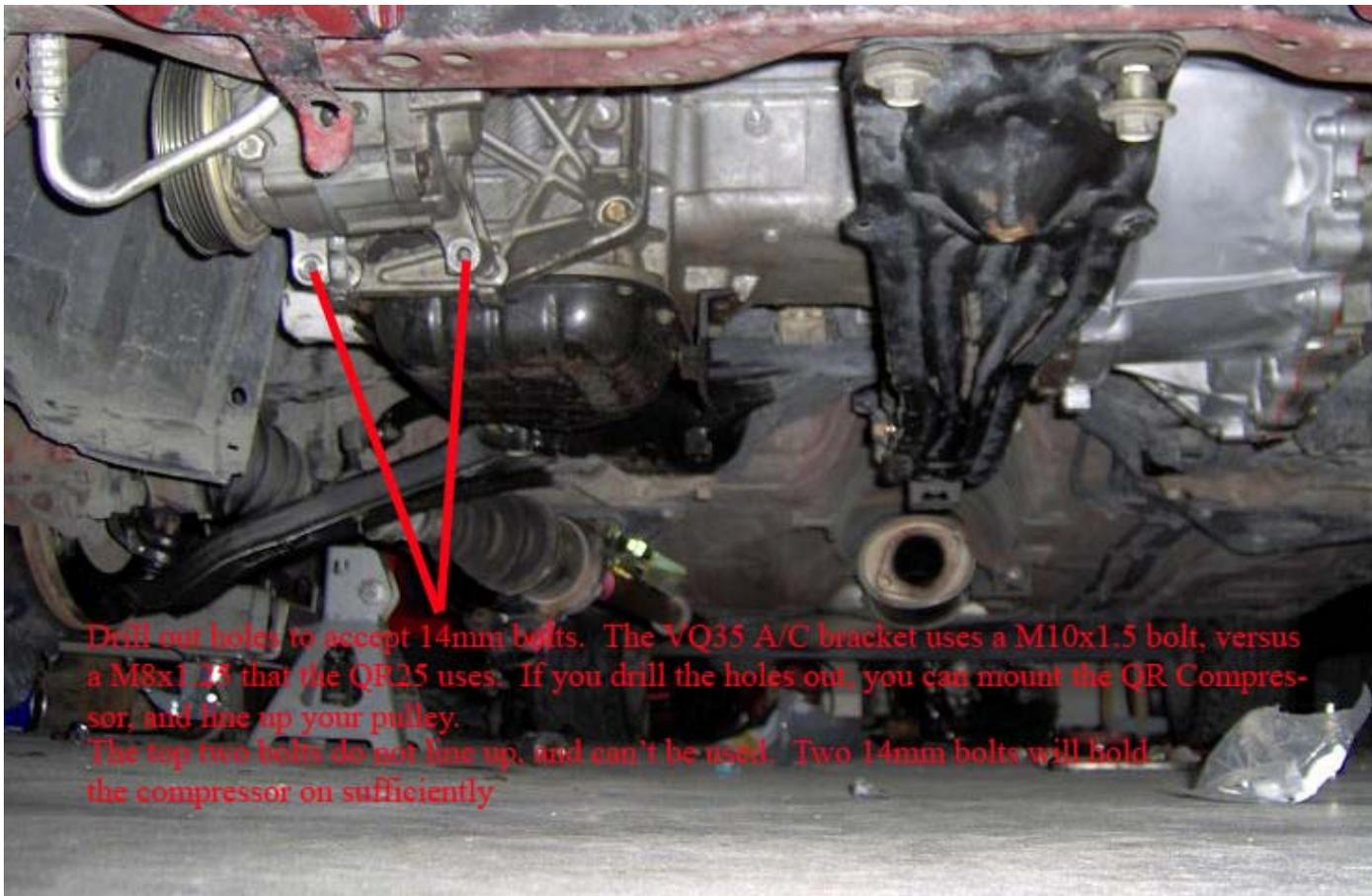
You will only be able to use those 2 bolts, but it will hold up just fine. Our test car has been running for almost 6 months with this setup. If you drill the holes slightly larger, you can line the pulley up better, so that you can use 6 rib belt, instead of 5 rib. Take your time, and line it up, and you will be fine. Tighten those 14mm bolts down tight, and use some Loc-Tite for added insurance.
