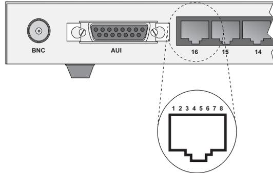
*Fig. A-1 RJ-45 Connector Pin Numbers*
