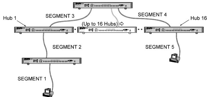
*Fig. 3-3 Horizontal Cascading*
