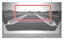
Switches between the front view camera and rear view camera each time you touch the illustrated area.
