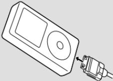
To disconnect the iPod, stop the playback by touching the [▶||] button on the source control screen, and then disconnect the iPod. See <Source Control Screen> (page 30).
