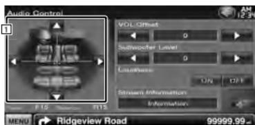
1 Adjusts the front/back and left/right balance of the volume by touching the Adjust screen.
