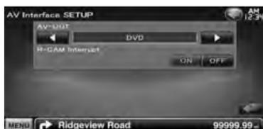
**[AV-OUT]** Selects an AV source to be output at the AV OUTPUT port. (☑ "AV-IN1")
