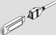
To disconnect the USB device, touch the [▲] button on the source control screen, and then disconnect the USB device. See <Source Control Screen> (page 23).
