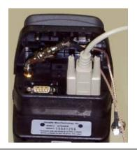
For real-time, sub-meter locations, attach the COM port cable to COM2, and the antenna cable to the connector as shown.
