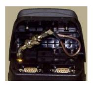
To use the Alto-G12 without the real-time differential, use the built-in antenna as shown.
