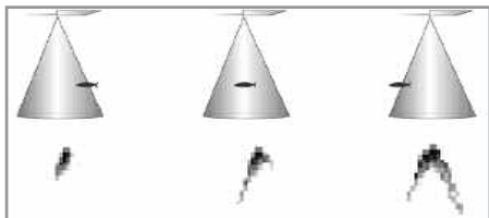
Transducer Cone and Fish Arches
