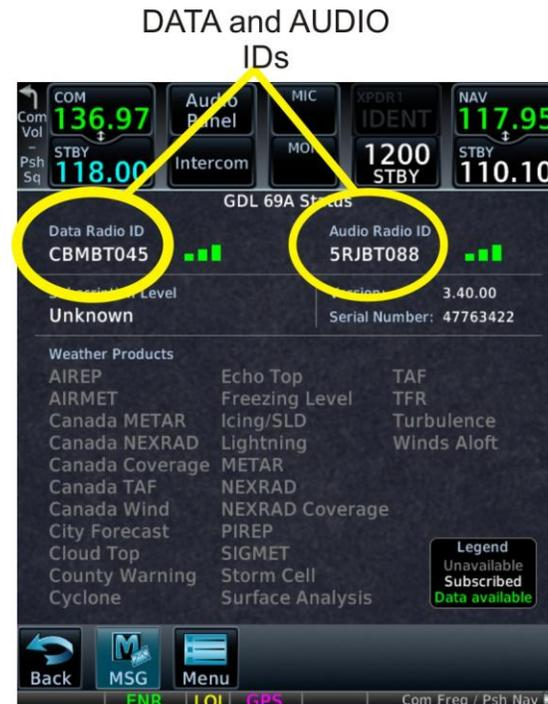
**Figure 8-1. GDL 69 Series Unit Data and Audio Radio IDs on Status Page**
