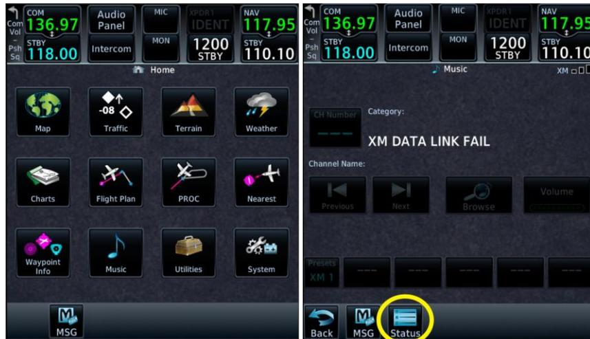
Figure 8-2. Accessing GDL 69 Series Unit Status Screen using 'Music' Key
