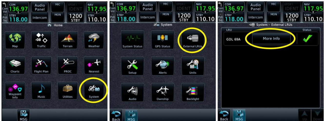
Figure 8-3. Accessing GDL 69 Series Unit Status Screen using 'System' Key
