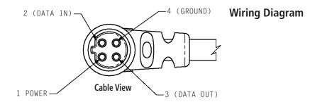
Interface formats are selected from the Setup 'Interface Page' on page 55 of this manual. See also page 68 for using the Rino with MapSource. The input/output lines on your Rino unit are RS-232 compatible, allowing easy interface to a wide range of external devices, including PC's, differential beacon receivers, marine autopilots and /or a second GPS receiver.
