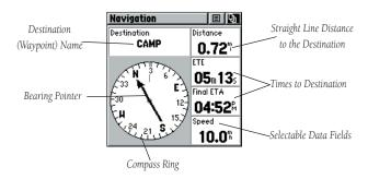
The Navigation Page provides active guidance with a rotating compass ring that shows your course over ground (track) while you're moving and a bearing pointer to indicate the current direction to your destination (bearing) relative to the course over ground.
