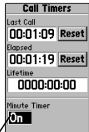
The Minute Timer Signals with 2 Short Beeps every 60 Seconds which cannot be heard by Other Parties.
