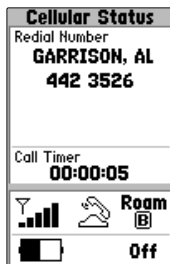
Cellular Status Page Displaying a Redial Number, Call Timer and "In-Use" Indicator
