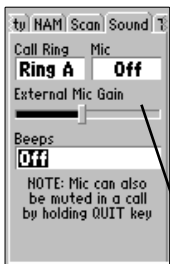
The 'External Mic Gain' feature is used with the Vehicular Adapter Kit
