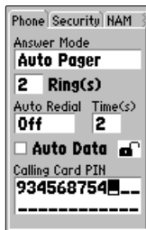
Padlock icon open and PIN field open for PIN entry. After entry, close padlock icon and the field will be closed to viewing.
