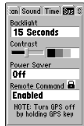
Remote Command can be enabled or disabled and is protected by a security password
