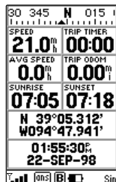
Position Page with simulated data. Note "Sim" indicator on right side of Status Bar
