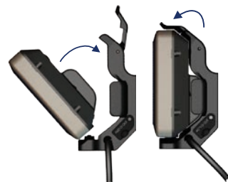
Placing the GPSMAP 640 in the Mounting Bracket
