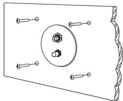
The GPSMAP 182/182C/232 with external antenna can be flush mounted on a flat panel of .08-.52" thickness using the cam lobe feature on its gimbal mounting bracket. When flush mounting the GPSMAP 182/182C/232, be sure to choose an appropriately sized location for the unit (see unit dimensions pg. 83) and leave 1.25" (32mm) clearance below the data card slot for inserting/removing data cards. For flush mounting the GPSMAP 232 unit, skip to the next set of instructions.
