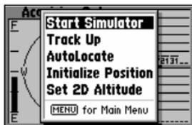
Select 'Start Simulator' from the Satellite Status Page to enable the built-in simulator.
