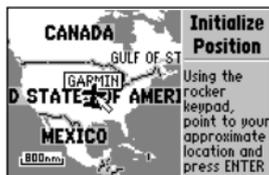
To initialize the GPS III, designate your approximate location directly on the map display. Use the rocker keypad and IN/OUT zoom keys to position the cursor on the map.
