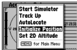
'Initialize Position' is used to designate your approximate position directly on the map display. The receiver uses this information to determine which satellites should be in view.
