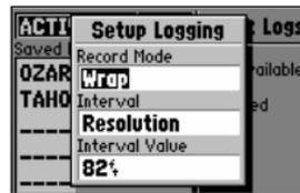
The 'Setup Logging' option allows you to change the criteria used to record the active track log.
