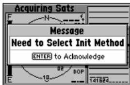
*When new (or if a position cannot be determined after 10 minutes), the GPS III will prompt you to initialize the receiver. The unit needs a starting position to determine which satellites are in view.*
