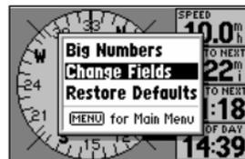
The 'Change Fields' option allows you to select from a list of available data types. Four different items may be displayed on the Compass Page—two when using the 'Big Numbers' option.
