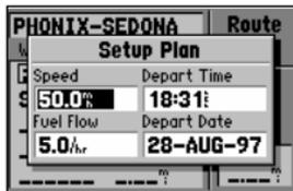
With the Route Plan Page displayed, use the LEFT/RIGHT keys on the rocker keypad to select the trip planning features. Press MENU and select 'Setup Plan' to define departure time, fuel usage and speed.
