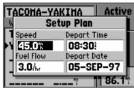
'Setup Plan' allows you to define planned speed, fuel flow and departure time in order to review trip planning figures.
