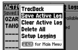
Select 'Save Active Log' to save the active log data for future use. This process extracts the most significant points along the active route (up to 250) and creates a 'saved log'.
