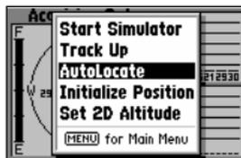
'AutoLocate' forces the receiver to search for all satellites (twelve at a time) until enough satellites are found to determine a position.
