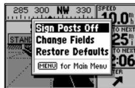
The 'Sign Posts Off' option allows you to remove the waypoint markers from the highway display.
