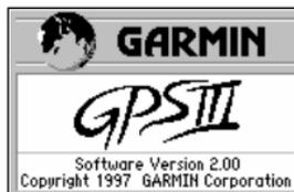
The Welcome Page is displayed when the GPS III is first turned on. After a brief self-test, it is replaced by a warning page for about 10 seconds. To skip the warning page, press ENTER.
