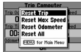
The trip odometer, trip timer and average speed readings can all be reset from the 'Trip Computer' option on the Main Menu. See page 66.
