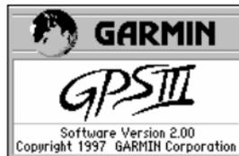
*The Welcome Page is displayed when the GPS III is first turned on. During this time the receiver is conducting a self test.*
