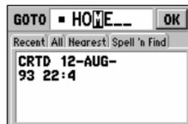
Press ENTER and use the rocker keypad to enter the identifier of the destination waypoint. Press ENTER to begin navigation.
